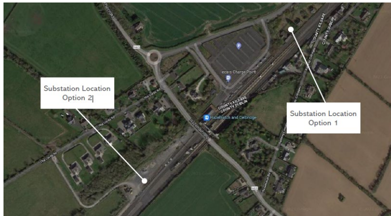
Figure 3-4 Proposed Hazelhatch Substation Locations
